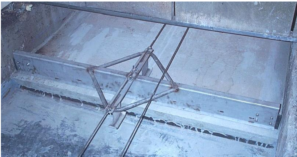
Figure 4. Scraper blade used for daily removal of manure from the pit. The manure pit has drains at both ends, through which the scraped manure was emptied to the sewer line.
